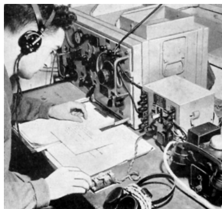
Wireless Remote Control Unit C allowed remote operation of Wireless Set No. 12 or No. 33. A Key and Plug Assembly No. 2B was issued with this unit (above).
