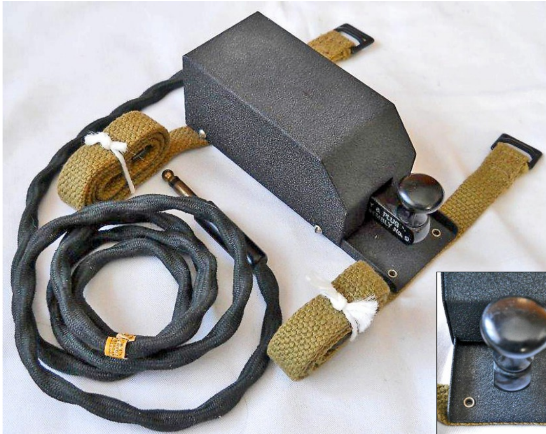
Key and Plug Assembly No. 9 ver. 9.1 was produced in the U.S.A. by J.H. Bunnell. Most significant differences to the British parent assembly were a type PL-55 plug and a smaller key knob.
