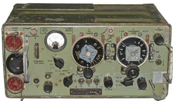
Wireless Set No. 19 (here shown the British Mk.III model, set without power supply unit). Use: primarily developed for AFVs but later used as a general purpose set. Frequency range 'A' set 2-8MHz; 'B' set 229-241MHz. MO control. R/T, MCW, CW. RF output 'A' set 1.2-2.5W (R/T). Range 'A' set up to 15 miles; 'B' set ¾ mile.
