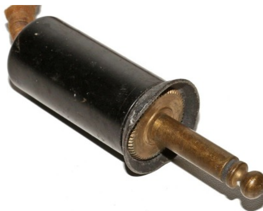
A black fibre disk protected the operator from coming into contact with high tension when inserting the key into the set key socket (above). This was an addition which was occasionally found fitted on other versions.
