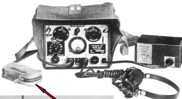
The Plug and Key Assembly No. 2B (Aust) issued with Wireless Set No. 208 Mk.II (above left) and 108 Mk.III (left) was carried in a waterproof cover (ZAA 8882).
