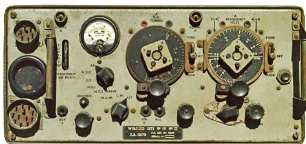
Wireless Set No. 19 (here shown the British Mk.II model, set without power supply unit). Use: primarily developed for AFVs but later used as a general purpose set. Frequency range 'A' set 2-8MHz; 'B' set 229-241MHz. MO control. R/T, MCW, CW. RF output 'A' set 1.2-2.5W (R/T). Range 'A' set up to 15 miles; 'B' set \frac{3}{4} mile.
